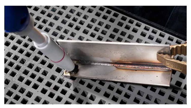
Electrochemical cleaning uses micro-arcs to remove welding residues from metal surfaces after welding and passivates the surface at the same time. For this purpose, a carbon fiber brush wetted with electrolyte at the ends is moved over the workpiece as more than one million micro arcs are generated.
